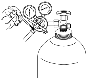
Figure 1. Testing Equipment For Leaks
