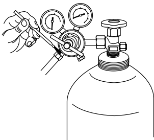
Figure 3. Testing Equipment For Leaks
