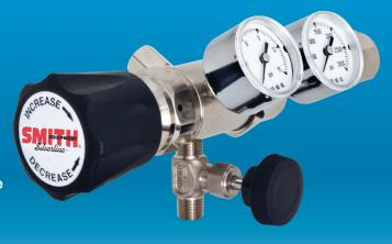
These two stage regulators are ideal where precise delivery pressure is critical in low flow applications of non-corrosive gases. The slim design makes it ideal for lab applications where space constraints exist. The design features include a stainless steel diaphragm in the second stage, brass piston first stage, capturable preset safety relief vent, sintered brass filters for added protection of internal components.
